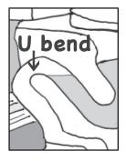
In 1775, the toilet got an upgrade. Someone invented a new kind of pipe bent in the shape of a U. Today, this pipe is called a U-bend. The pipe's bend is important because it traps the smelly water. This invention made people want a flushing toilet in their house.
